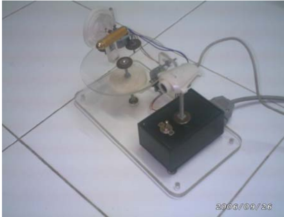
Fig3. Image processing based laser tracking system
