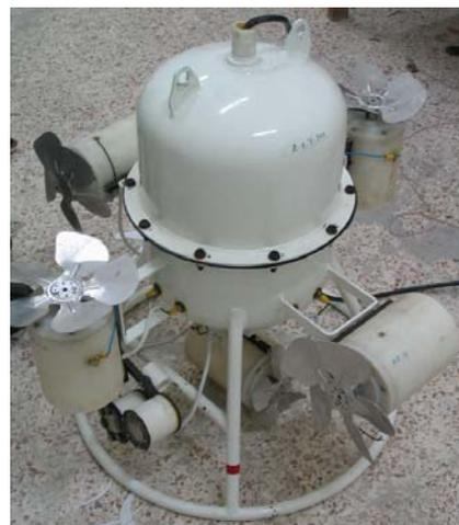
Figure 1: Underwater remotely operated vehicle constructed in Guilan University
