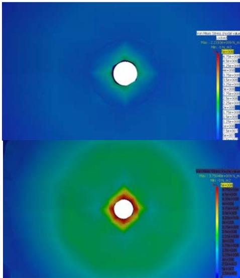
Figure 8 : Stress at the center of cylinder before and after modification
