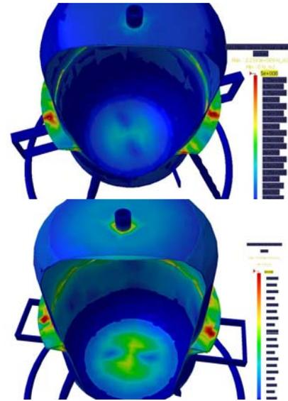
Figure 9 : Stress at the center of cylinder before and after modification in View of the center of bottom half body
