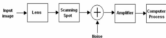
Fig 4 the elements of an image processing system
