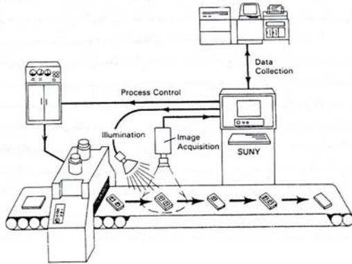
Fig1. A Typical Industrial Vision System
