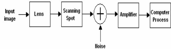
Fig5. The elements of an image processing system
